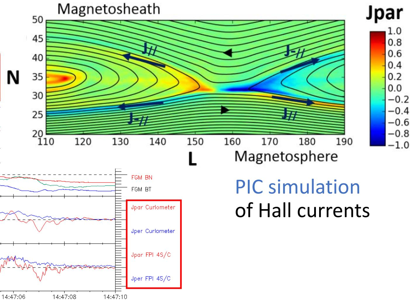
MMS currents confirm basic structure of Hall currents from simulations
